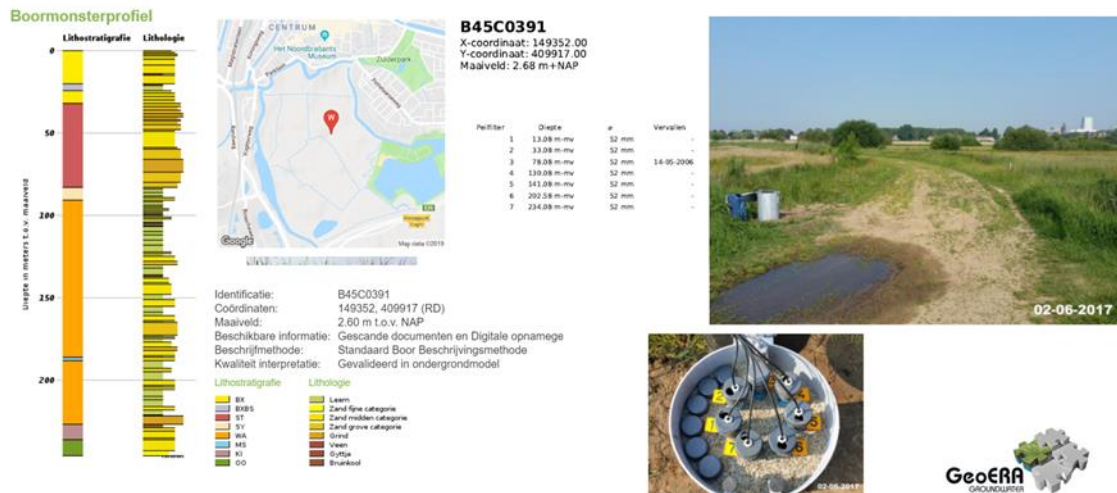
Figure 5.26 Borehole description, well construction and location of the observation well B45C0391, which contains 7 well screens of 52 mm diameter between 12 and 234 m depth.
