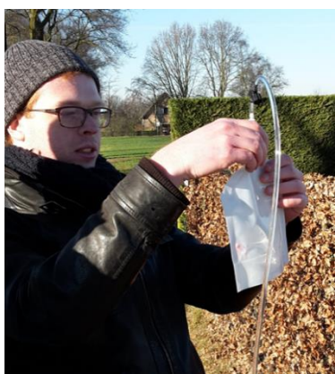
Figure 5.5 Sampling for dissolved gases in groundwater using Isoflasks
