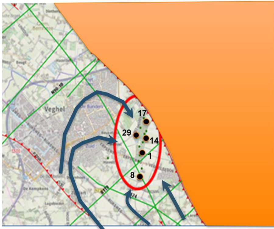
Figure 5.24 Conceptual model of the flow around the Veghel well field BW27. Lateral inflow from the east is limited to assumed sealing in the fault zone. Given their position in the center of the overall well field, the wells PP1 and PP14 are forced to pump a larger proportion of their water from deeper parts of the subsurface, whereas the pumping wells that are more at the fringe of the well field (PP8 and PP29) have easier access to water from the pumped aquifer and above.
