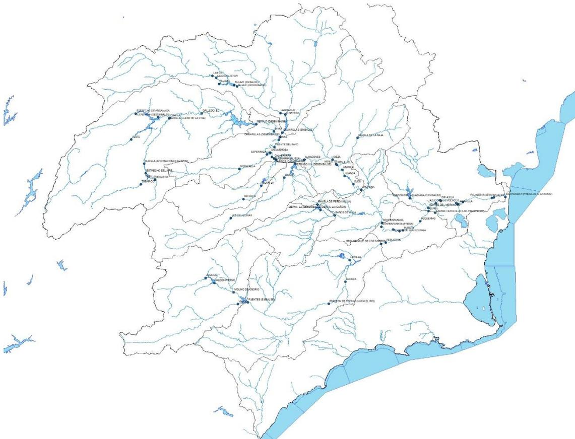
Figure 4.2. River subbasins and gauge stations to calibrate Temez model.
