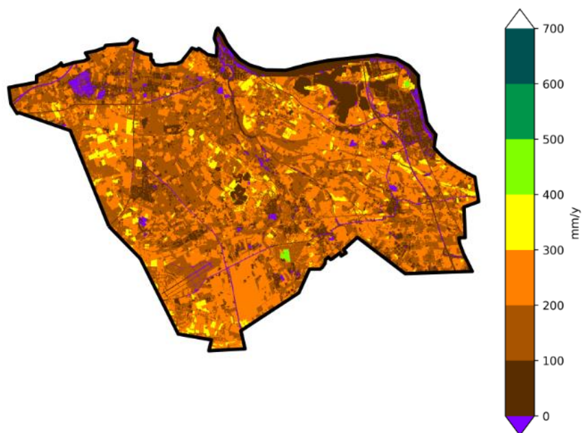
Figure 5.18. Average groundwater recharge in pilot area De Raam (mm/year) in period 2011-2018
