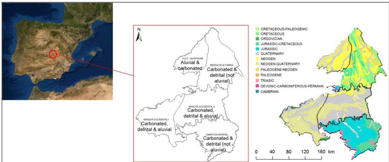
Figure 14: Groundwater bodies where COP methodology has been applied (left) and geology (right).
