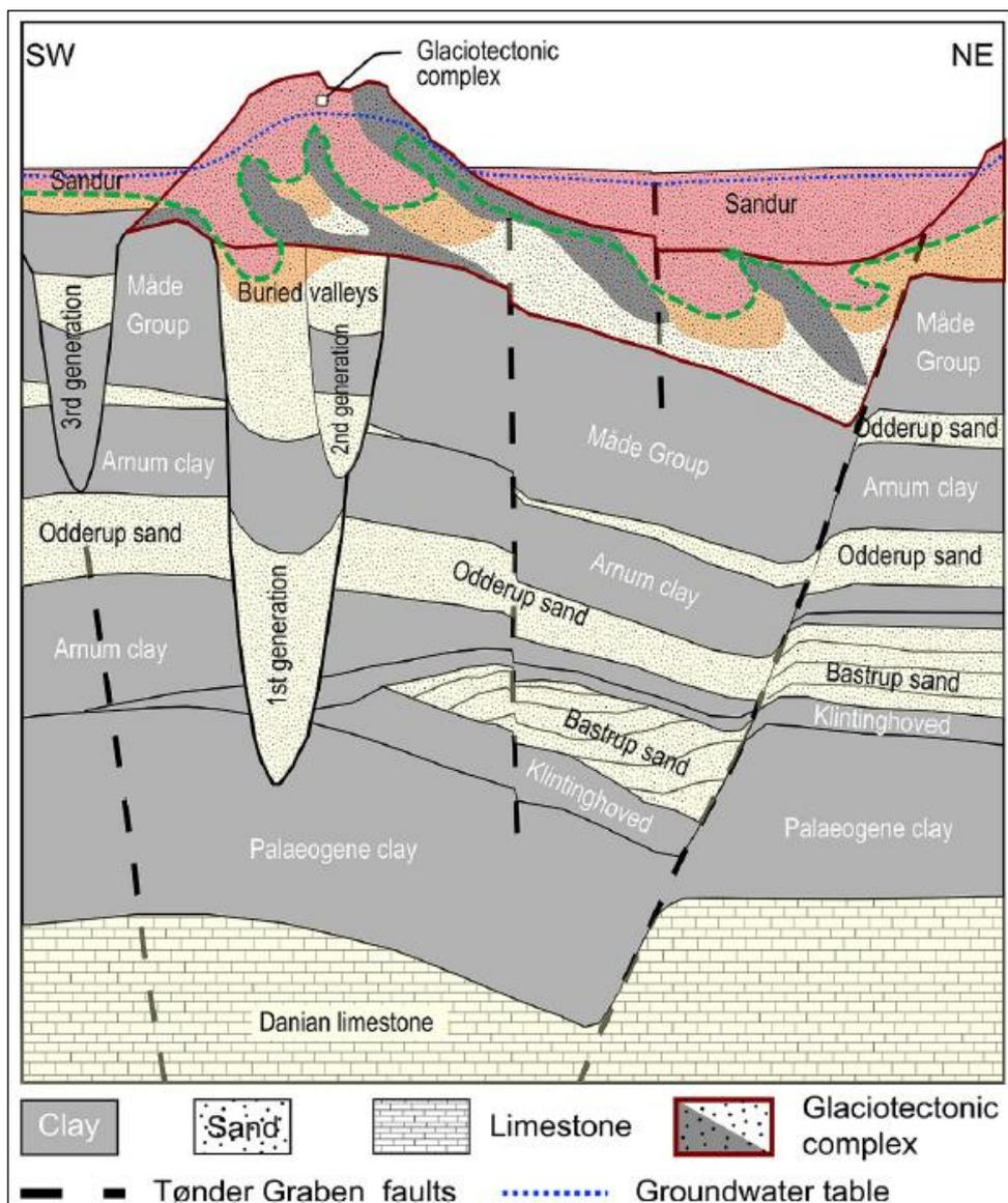
Figure 11: Conceptual diagram showing the geology in the Glaciotectionic complex with a complex redox architecture (conceptualised) and nitrate aquifer vulnerability (modified from Hansen et al. (2016, 2015).
