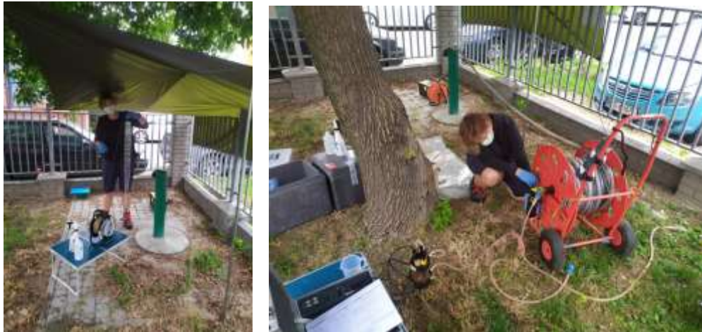
Figure 5: Taking water samples with a discrete sampler and with a submersible pump.
