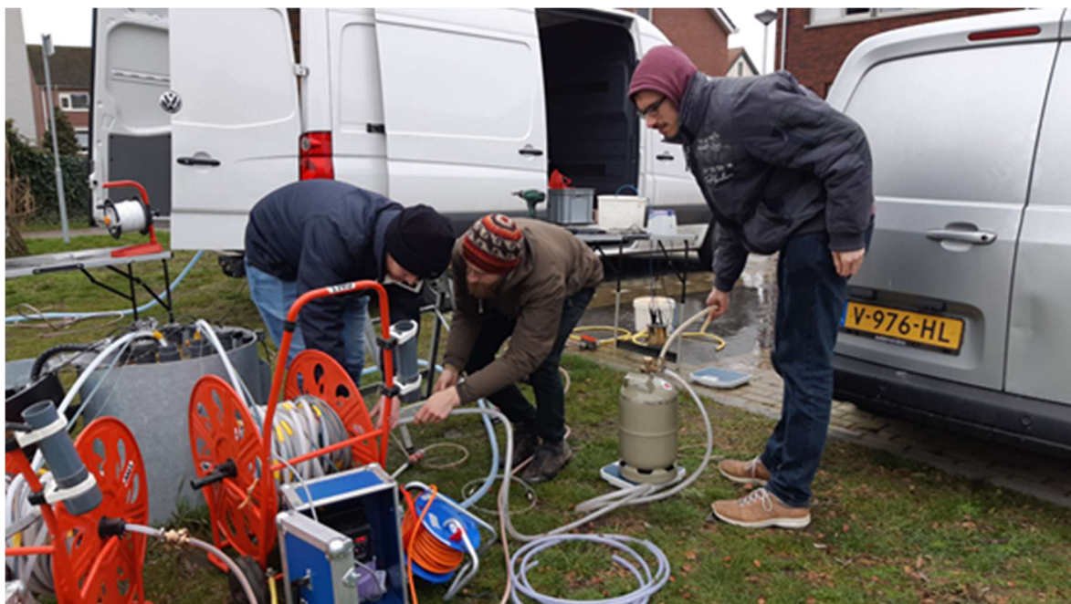
Figure 3.4 Sampling for noble gases and ^{39}\text{Ar} around BW10
