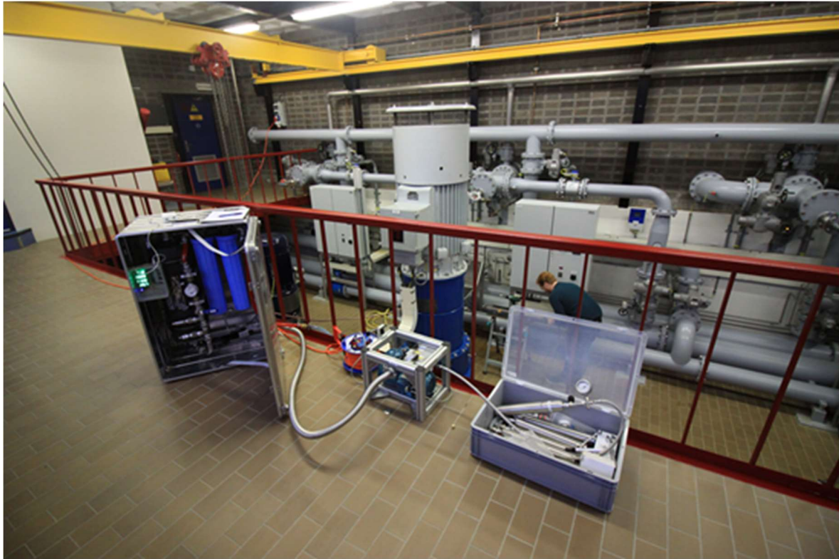
Figure 3.5 Sampling water from a 'raw water branch' for ^{39}\text{Ar} with the new contactor setup (left). Gas samples were compressed and stored in stainless steel cylinders (right) using a combined vacuum/compression pump (middle).
