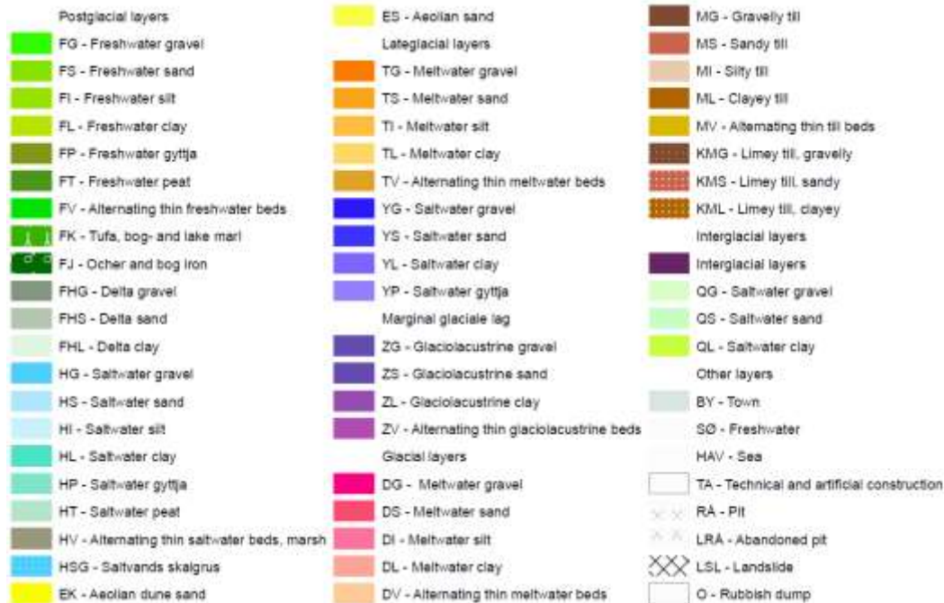
Figure 2: Selection of Gravesen & Fredericia's (1984) codes used in the Surface Geology Map of Denmark (1:25.000, version 4).
