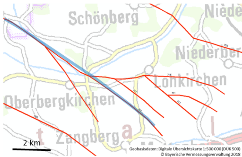
Figure 2: Horsetail splay structure at the southeastern end of Velden Fault , the smoothed fault traces (red) refer to the top of Upper Jurassic reservoir. Such branching out at the termination of faults could be fairly common, but is detectable in high-resolution up-to-date 3D seismic surveys only. The blue line represents the “pre-HotLime” trace of Velden Fault, as modelled based on legacy seismic surveys.
