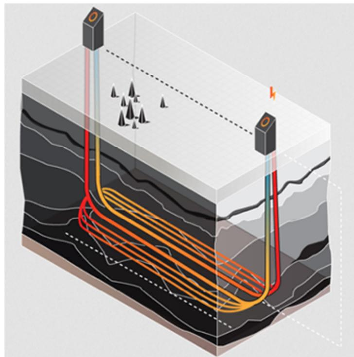
**Figure 6.7.** Eavor-Loop™ (Eavor Technologies Inc., [www.eavor.com](http://www.eavor.com)) as planned for implementation at the Geretsried Project drill site at about 2,600 m depth using the existing drill hole of GEN-1 and a new one at a sufficiently distant location.
