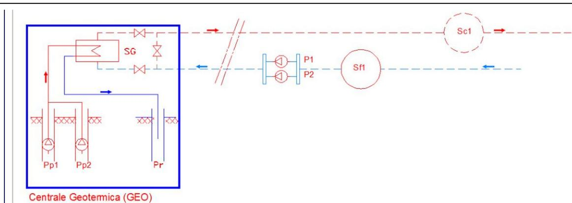
**Pp1 Withdrawal well n° 1  $Q_{\text{max}} = 200 \text{ m}^3 \text{ h}^{-1}$   $t_p = 102 \text{ }^\circ\text{C}$**
