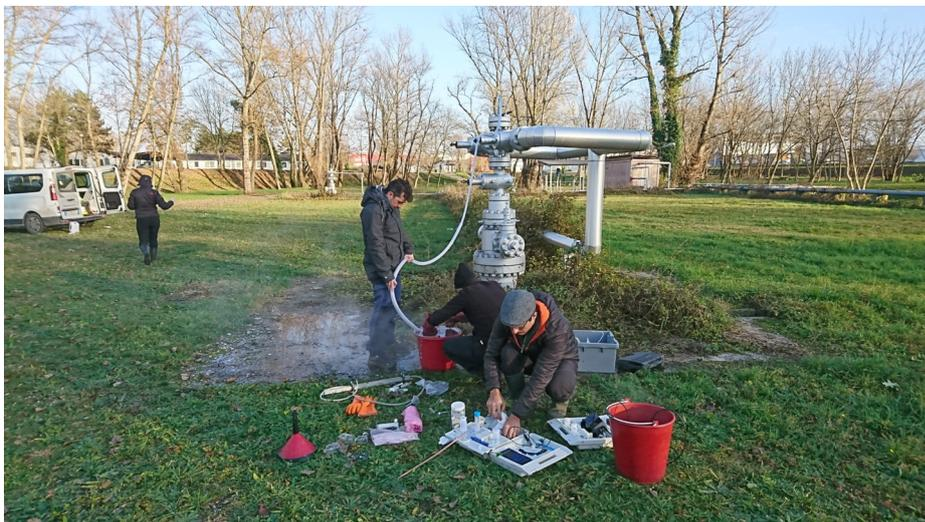
Figure 3.3. Water and gas sampling at the KBNZ-1b inactive production well of the ZGF (photo by V. Cazin).
