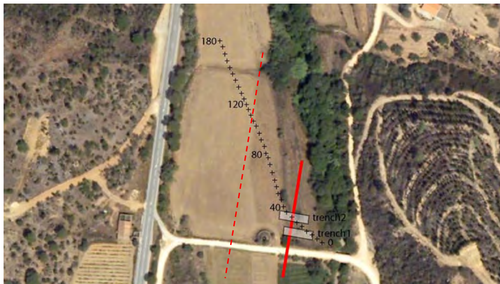
Figure 5.6 – Localization of the geoelectric tomography profile and trenches open at Framangola alluvial plain. The fault trace recognized through geomorphology is also indicated. Another fault trace inferred by the geoelectric tomography is indicated by the dashed line.
