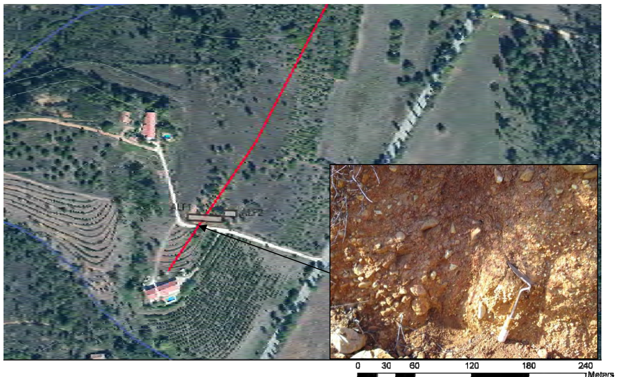
Figure 5.2 - Localization of trenches ALF1 and ALF2 at Barranco da Vaca site. The fault trace is indicated by the red line. The inset presents a detail of the coarse deposit contact with the medium sands is also included in the figure.
