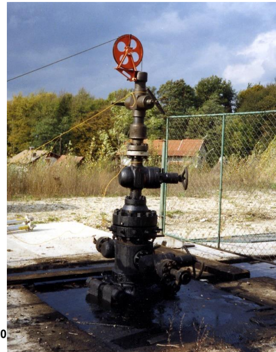
Fig. 1. Thermogram and photo of the deepest borehole in Slovenia, LJUT-1/88 in Ljutomer, from which also many cored rock specimens have been measured on thermal conductivity and HFD determined. The well is now liquidated.
