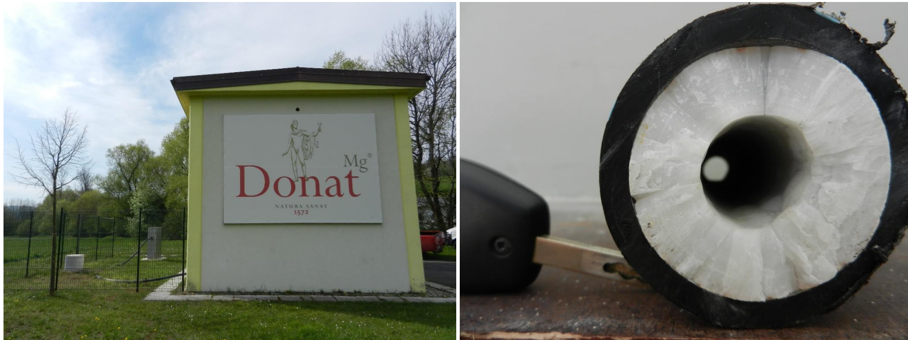
Fig. 1. Left: Degassing unit at the artesian well V-3/66-70 in Podplat. Right: This mineral water has very high scaling potential. When CO 2 is degassed at the surface, carbonate minerals (e.g. aragonite) precipitate in pipes, so they have to be periodically cleaned and/or replaced.
