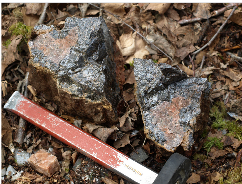
Figure 11. Field image of 10cm-sized lumps of Y-HREE-rich silicates, chiefly yttrialite-(Y) and presumed keiviite-(Y), from the Holmtjärn granitic pegmatite quarry, Dalarna (6691409/514398). Photo: Erik Jonsson.
