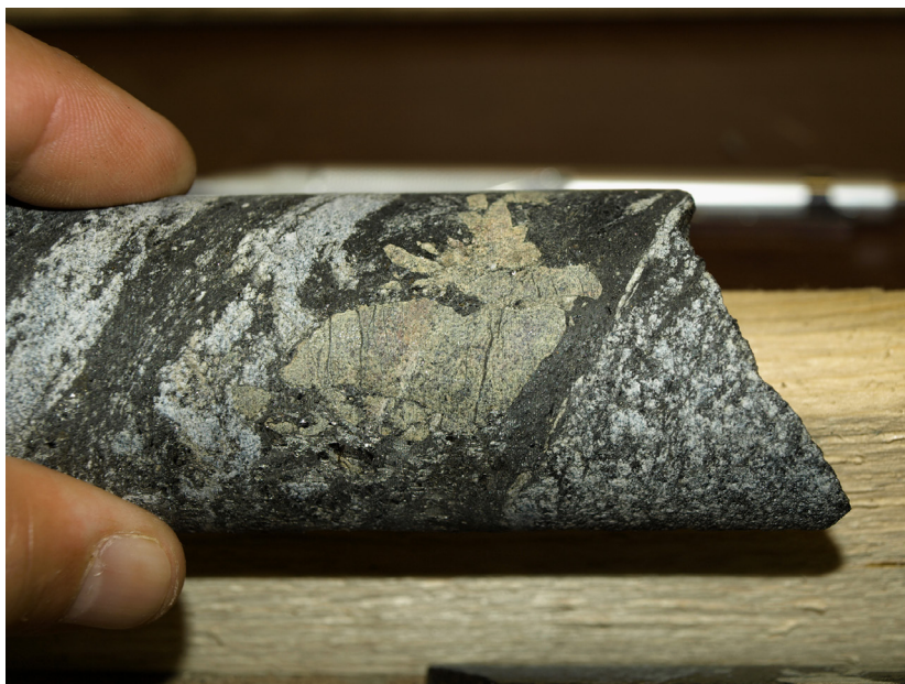
Figure 43. Coarse, subhedral yellowish crystal aggregates of monazite-(Ce) in a biotite-apatite-magnetite vein in a drill core from the former Tasman Metals resource in Olserum. Photo: Erik Jonsson.
