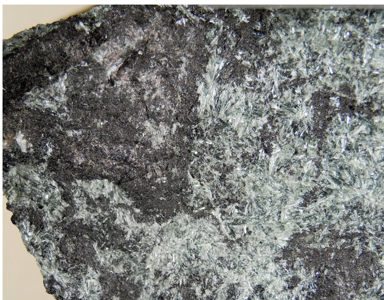
Figure 62. REE mineralisation at Rödbergsgruvorna: zoned veinlets of lighter, slightly pinkish-red cerite-(Ce) rimmed by black ferriallanite-(Ce), in a light green amphibole skarn. Photo: Per Nysten.
