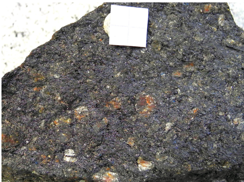
Figure 68. Hand specimen image of a fine-grained magnetite ore with abundant, subrounded feldspar clasts or crystals. The scale bar in the upper part of the image is 2 cm wide. Sveafallen (6563296/467479). Photo: Per Nysten.
