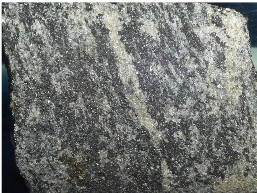
Figure 37. Banded apatite-magnetite ore from the Grängesberg Export field. Section of drill core, image width approximately 5 cm. Photo: Erik Jonsson.
