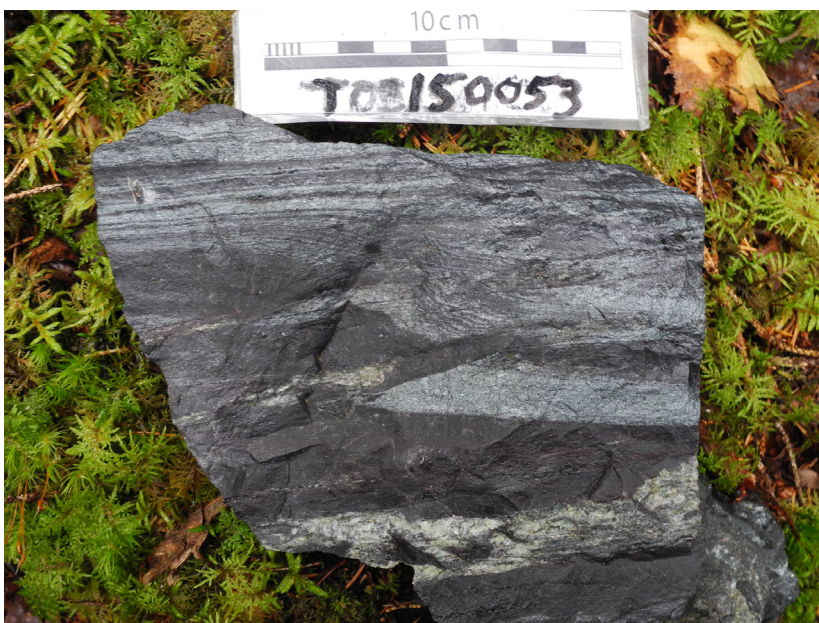
Figure 54. Amphibole skarn-bearing magnetite-hematite banded iron ore from Stora Högforsgruvan (6636536/534256). Photo: Torbjörn Bergman.
