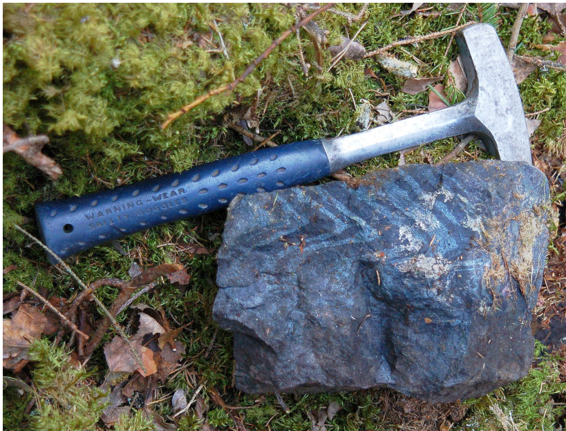
Figure 53. Hematite-metachert-dominated banded iron ore (BIF) exhibiting chevron-style folding; dump sample at Stora Högforsgruvan (6636536/534256). Photo: Erik Jonsson.
