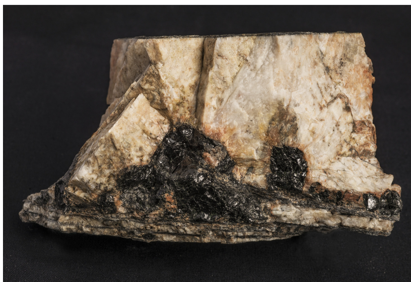
Figure 10. Hand specimen featuring subhedral black crystals of gadolinite-(Y) up to approximately 2 cm, associated with platy aggregates of biotite (subhorizontal aggregates in the lowermost part of the specimen) and pale feldspar, from the Ytterby pegmatite quarry on the island of Resarö, west of Vaxholm (6592332/690226). Photo: Carl-Erik Alnavik.
