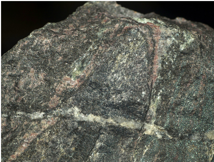
Figure 48. A folded and recrystallised reddish band of REE silicates (reddish tone from abundant cerite-(Ce), in addition to the presumed Fe analogue of västmanlandite-(Ce), for example) within the banded iron formation mined at (Stora) Högfors (6636536/534256), north-northeast of the Bastnäs field. The folded REE silicate band was later cross-cut (and slightly displaced) at a high angle by a quartz vein (subhorizontal in this image), which contains minor ordinary allanite-(Ce). Photo: Erik Jonsson.
