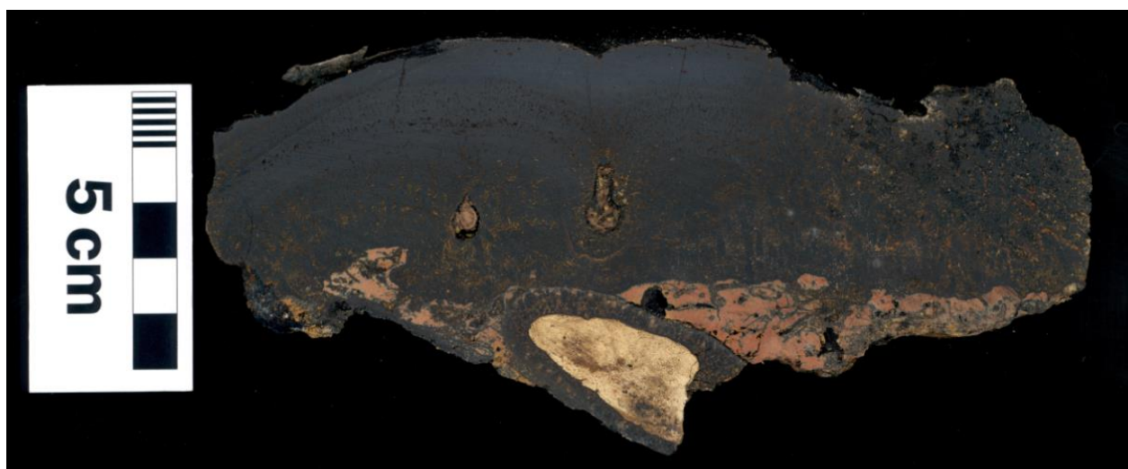
Cross section of a cobalt-rich Fe-Mn crust from the Canary Islands. Photo: IGME.
