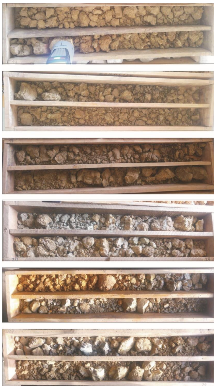
Figure 4: Photographs of archival Bobolice B-4 drilling cores (interval 14-25 m) tested for geochemical analyzes by use of portable XRF spectrometer in FRAME WP7 works.
