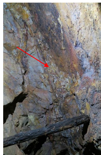
Figure 5: Approximately 1 m wide Baryte ore vein in the »Main Transport Adit«
