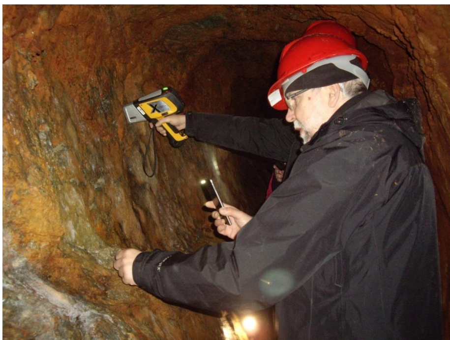
Figure 2: Rock examinations by used of portable XRF inside the historical tin mine of St. Leopold in Krobica (Sudetes, NE part of Bohemian Massif).
