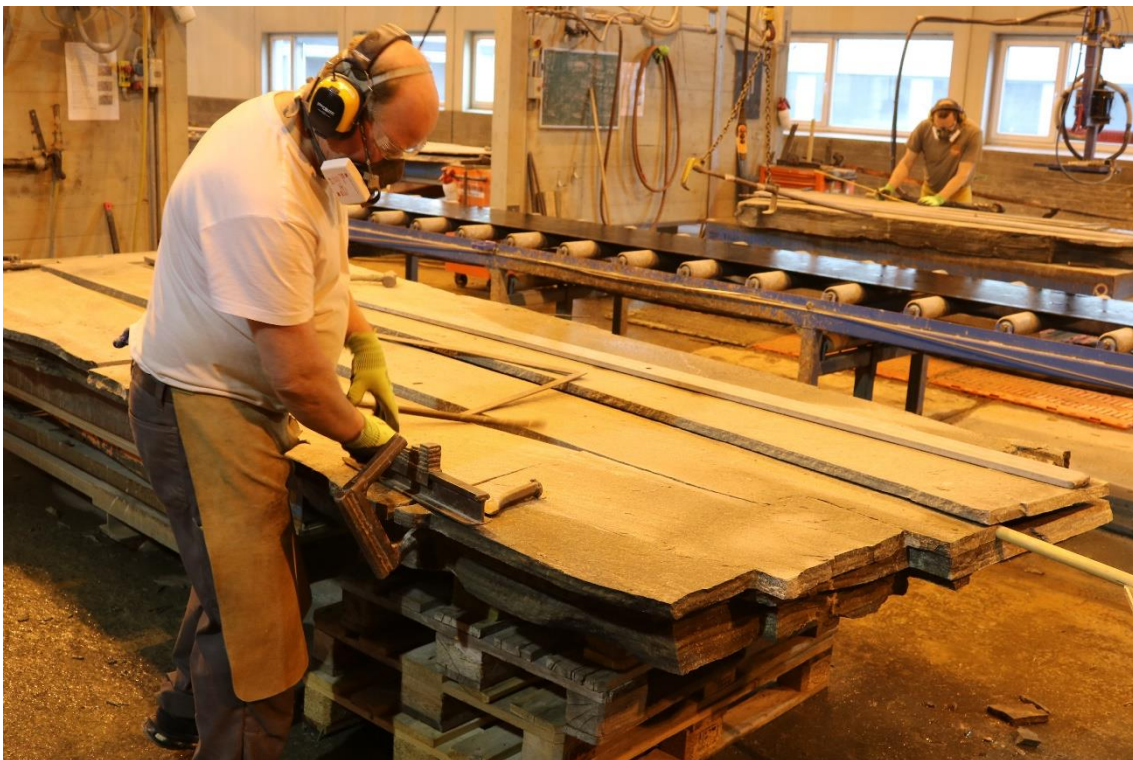
Figure 4. Traditional breaking of schist slabs, Oppdal, Norway
