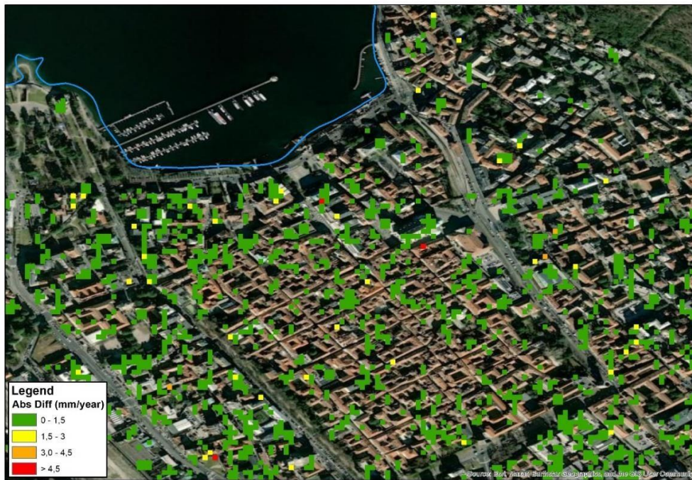
Figure 5: Example of spatial validation of velocities. Pixels without InSAR data in both datasets have been removed because the triggering phenomenon is not identified and
