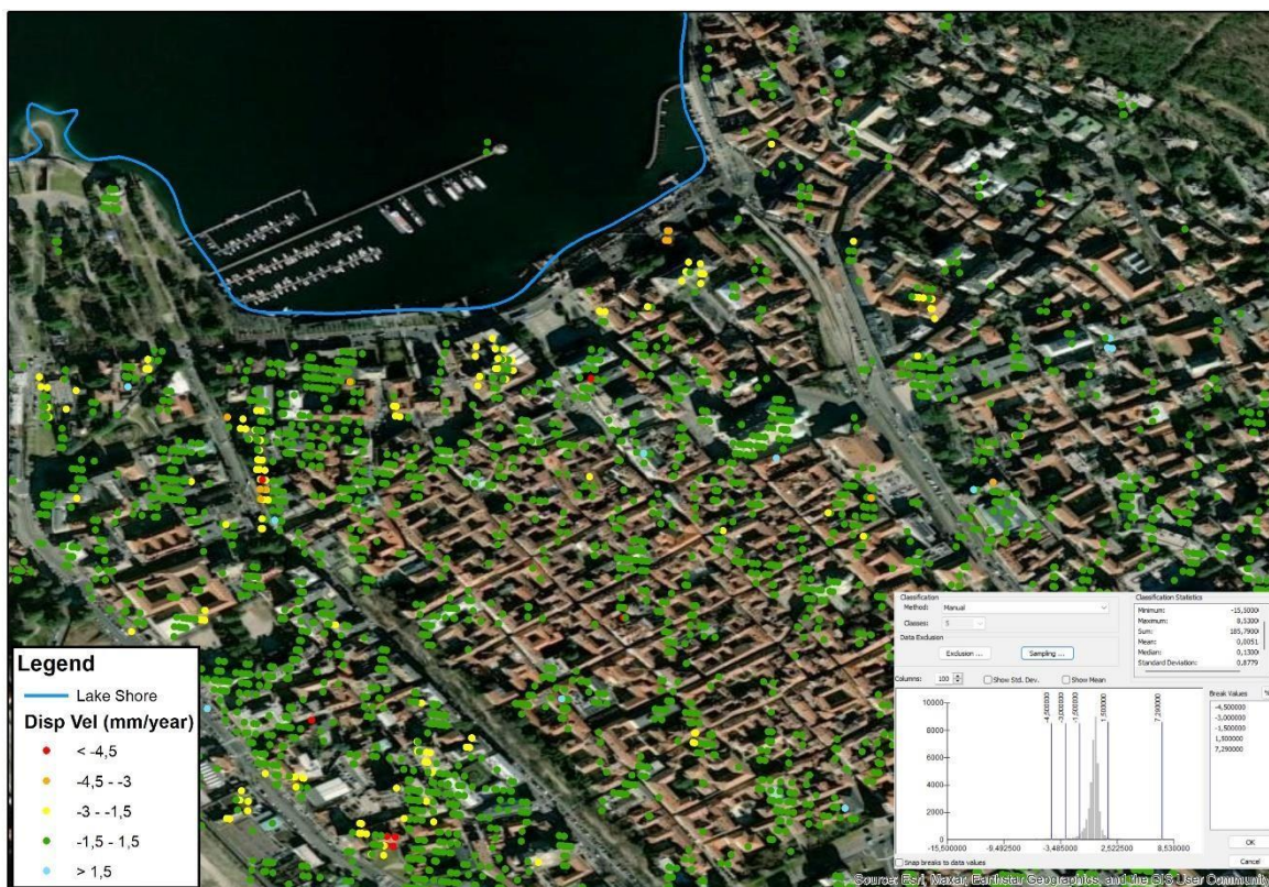
Figure 4: Mean LOS displacement velocities (PSIG). Sentinel-1, March 2015 – February 2022
